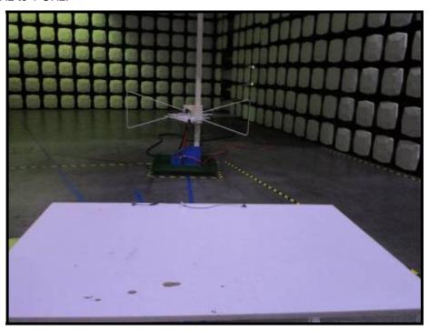
Above 1 GHz: (full anechoic chamber)
