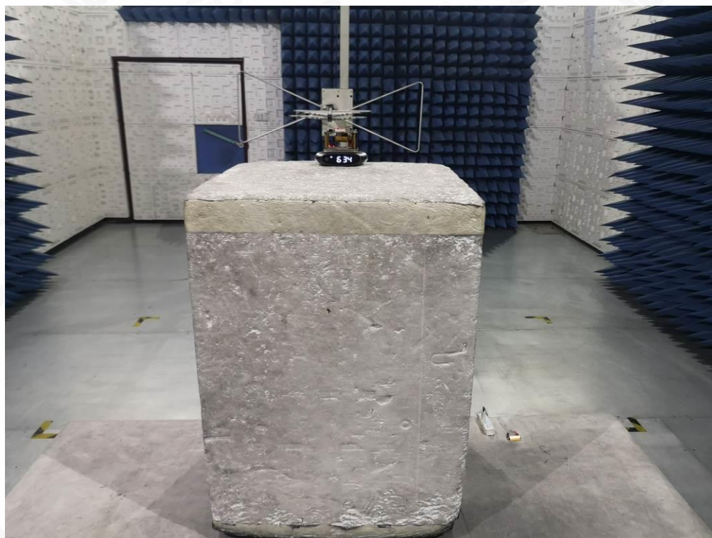
FCC RADIATED EMISSION TEST SETUP 30MHz-1GHZ
