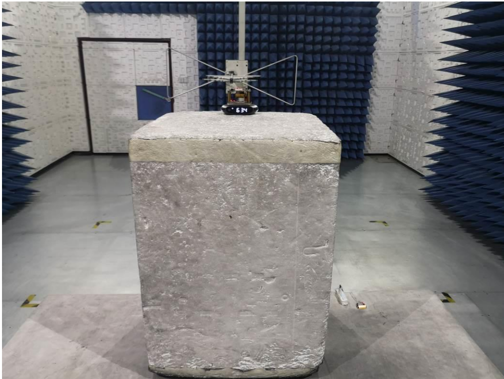
FCC RADIATED EMISSION TEST SETUP 30MHz-1GHZ
