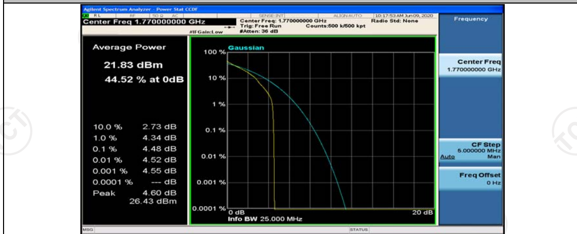
(Channel Bandwidth:20 MHz)_HCH_QPSK_1RB#49
