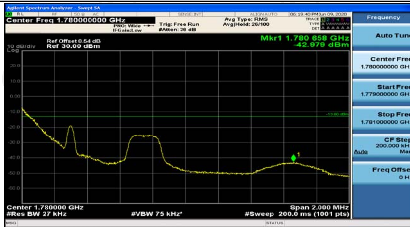
(Channel Bandwidth: 1.4 MHz)_HCH_QPSK_1RB#3
