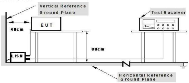
Note: 1. Support units were connected to second LISM. 2.Both of LISNs (AMN) are 80 cm from EUT and at least 80 from other units and other metal planes
