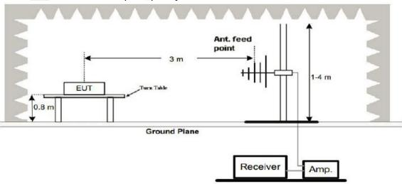
3. Radiated Emission Test-Up Frequency Above 1GHz
