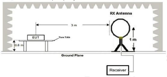
2. Radiated Emission Test-Up Frequency 30MHz~1GHz
