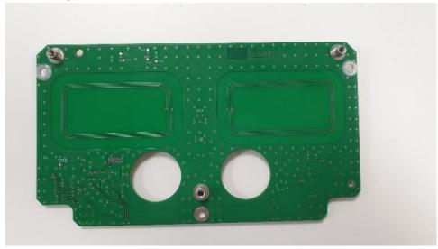
RMCIJ1 is a RFID module integrated in Markem-Imaje CIJ printers which ensures the authenticity and reliability of ink and additive cartridges
