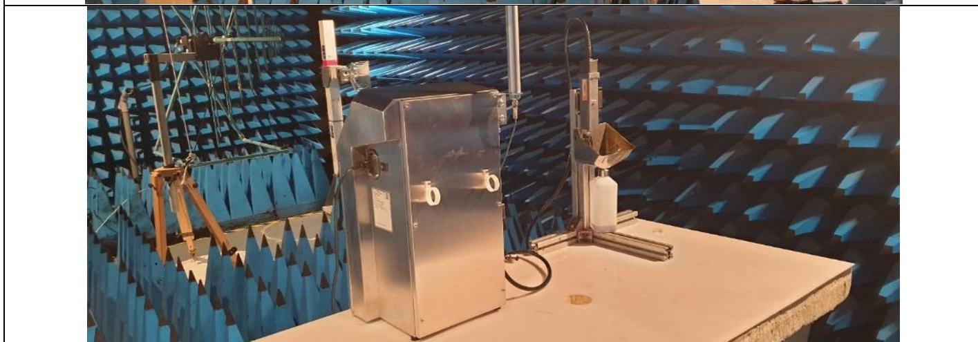
Test setup in anechoic chamber – Frequency <1GHz
