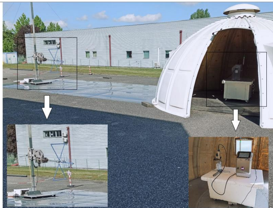
Photo Setup – OATS (Bilog antenna)
