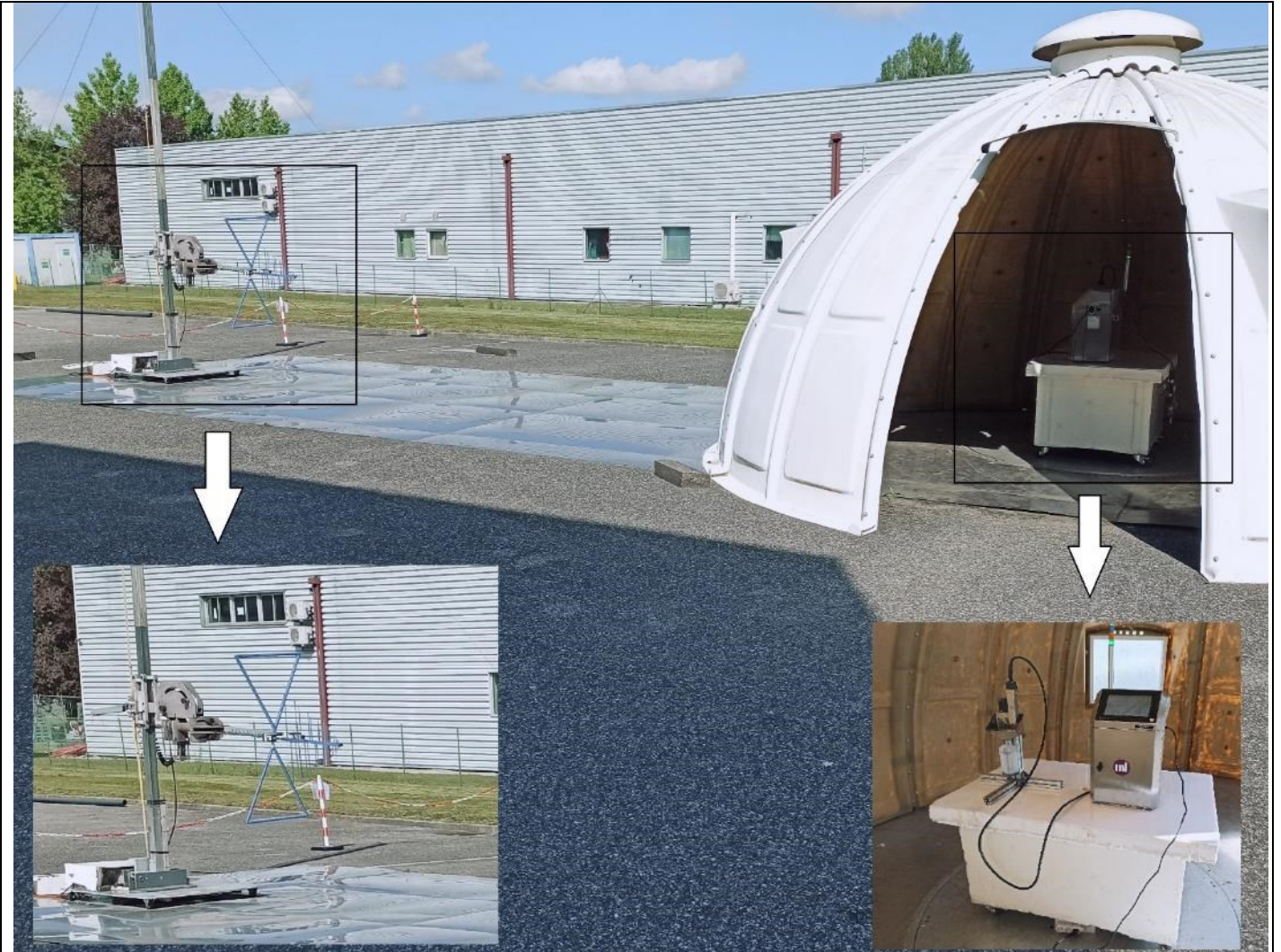
Photo Setup – OATS (Bilog antenna)
