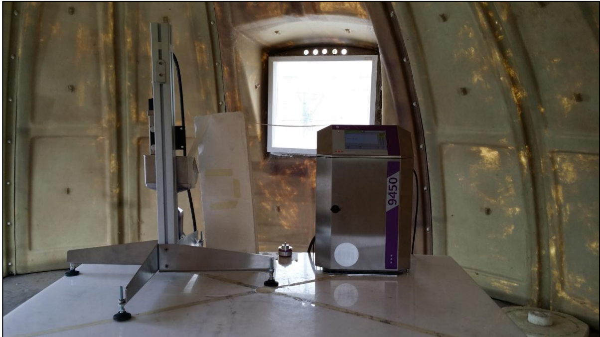
Radiated emission test setup
