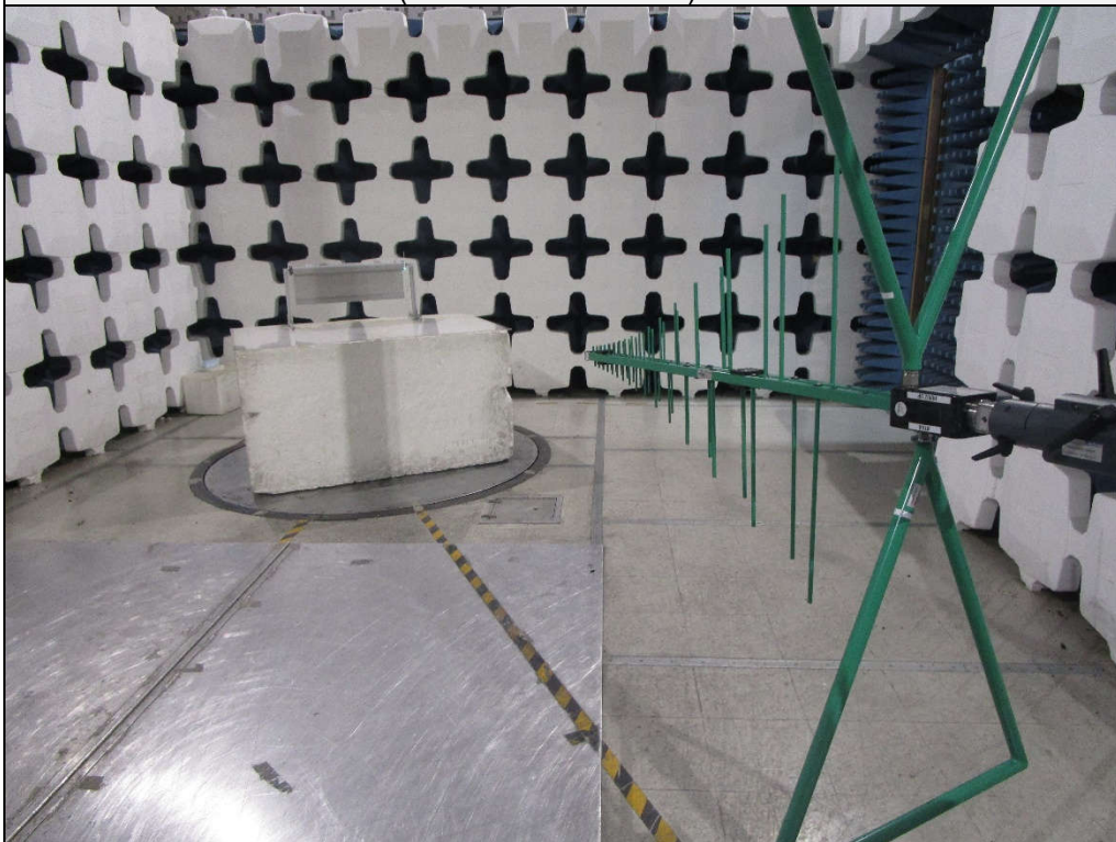
Test Setup for Radiated Emissions: 30MHz to 1GHz, Vertical Polarization (Roller Window Shade)
