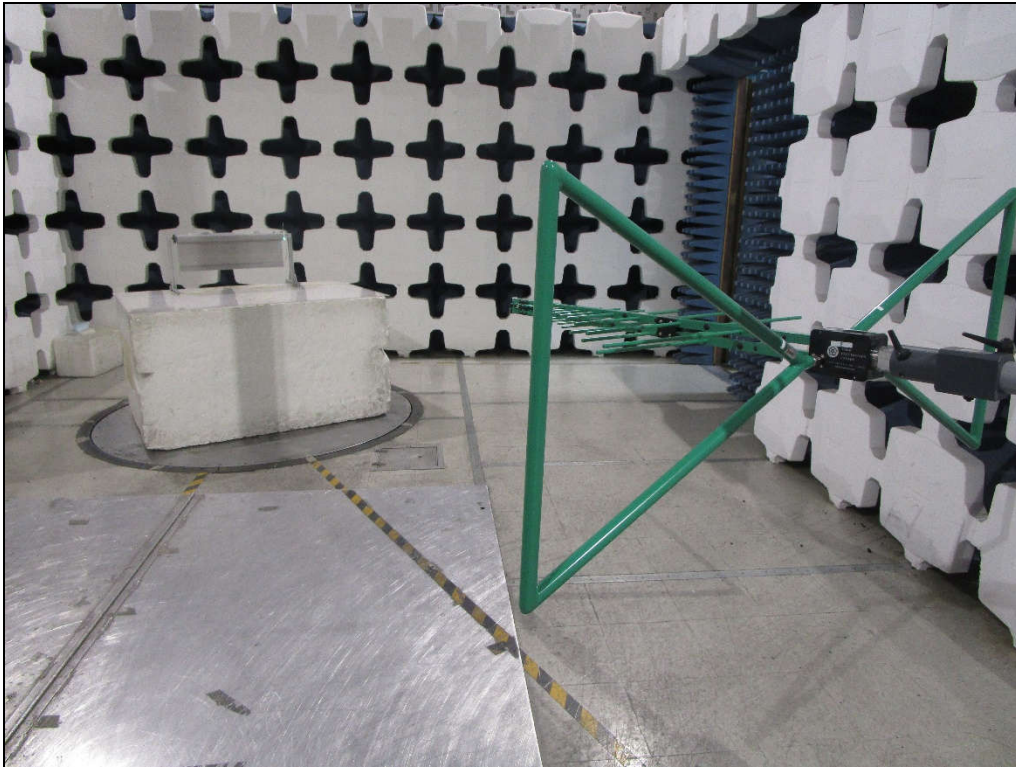
Test Setup for Radiated Emissions: 30MHz to 1GHz, Horizontal Polarization (Roller Window Shade)
