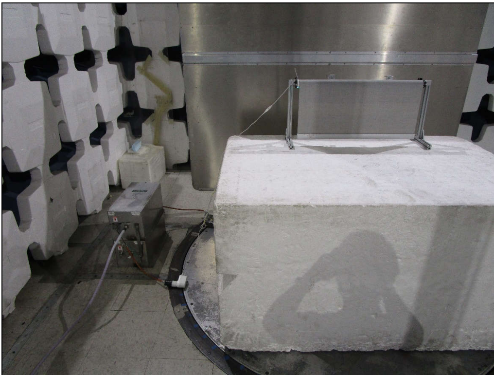
Test Setup for Powerline Conducted Emissions Test (Roller Window Shade)
