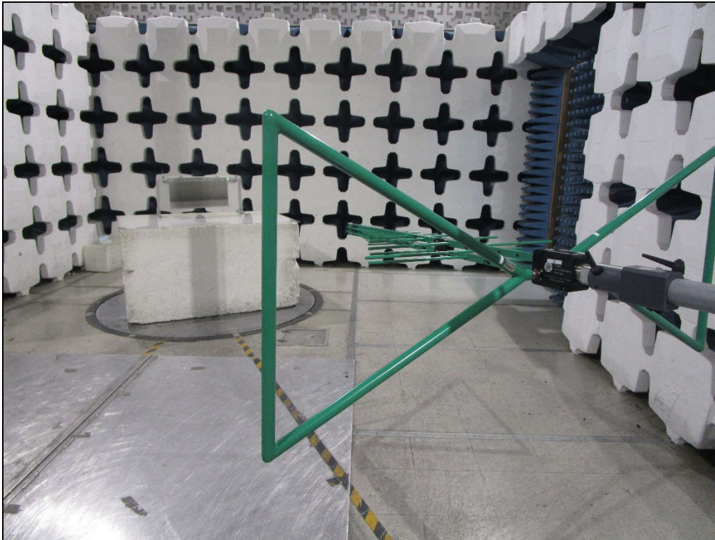
Test Setup for Radiated Emissions: 30MHz to 1GHz, Horizontal Polarization (Cellular Window Shade)
