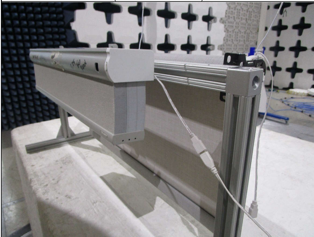
Test Setup for Powerline Conducted Emissions Test (Cellular Window Shade)
