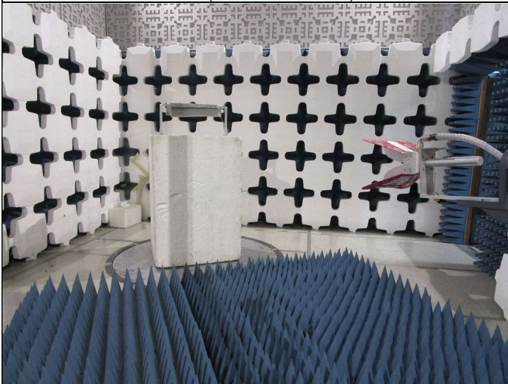
Test Setup for Spurious Radiated Emissions, Above 1GHz – Antenna Polarization Vertical (Cellular Window Shade)
