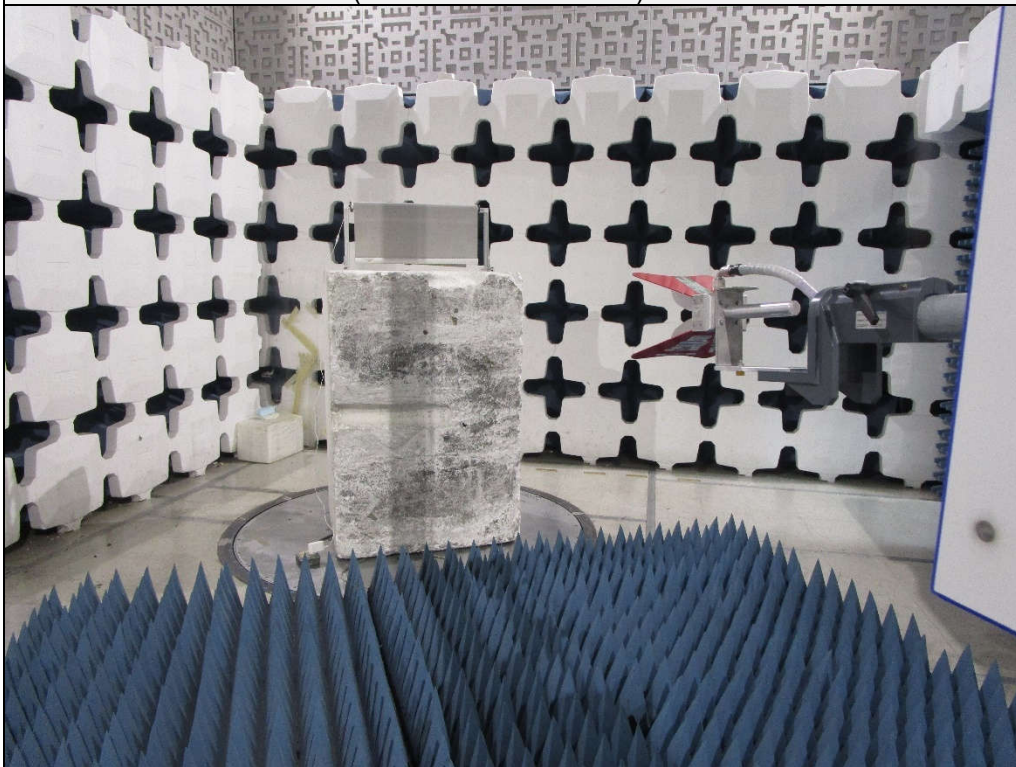
Test Setup for Spurious Emissions: Above 1GHz, Vertical Polarization (Cellular Window Shade)
