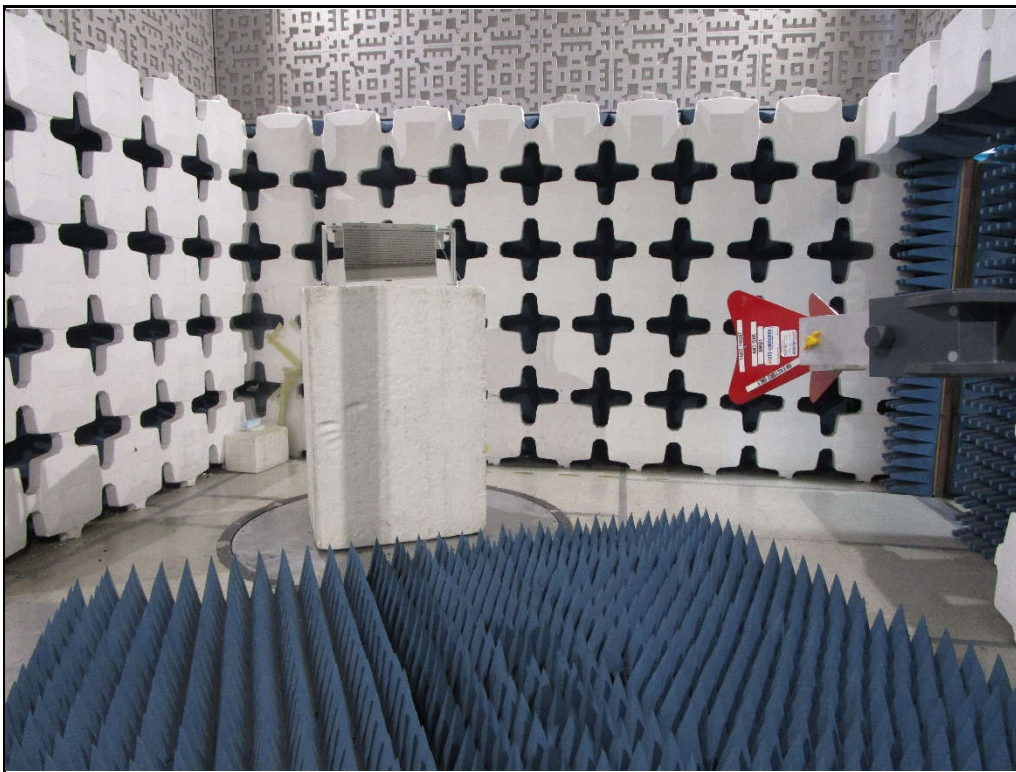
Test Setup for Spurious Radiated Emissions, Above 1GHz – Antenna Polarization Horizontal (Cellular Window Shade)
