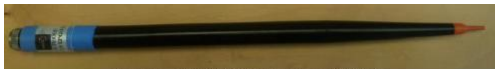
Figure 1 – MVG COMOSAR Dosimetric E-field Dipole
