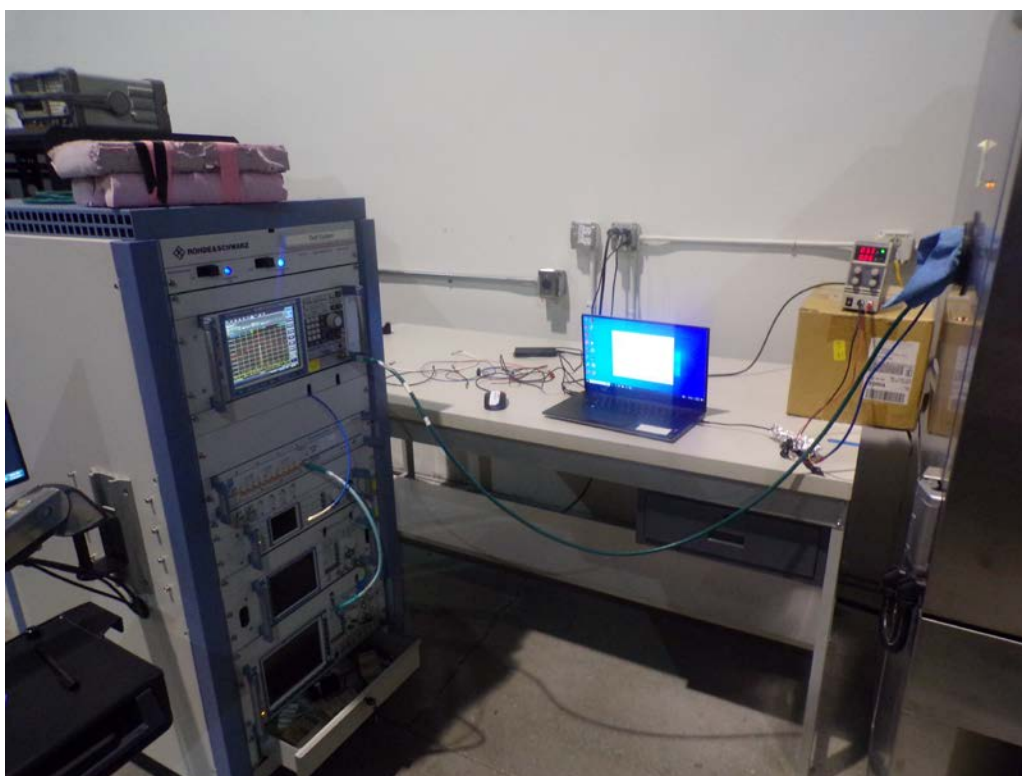
Frequency Stability – Outside Chamber Setup
