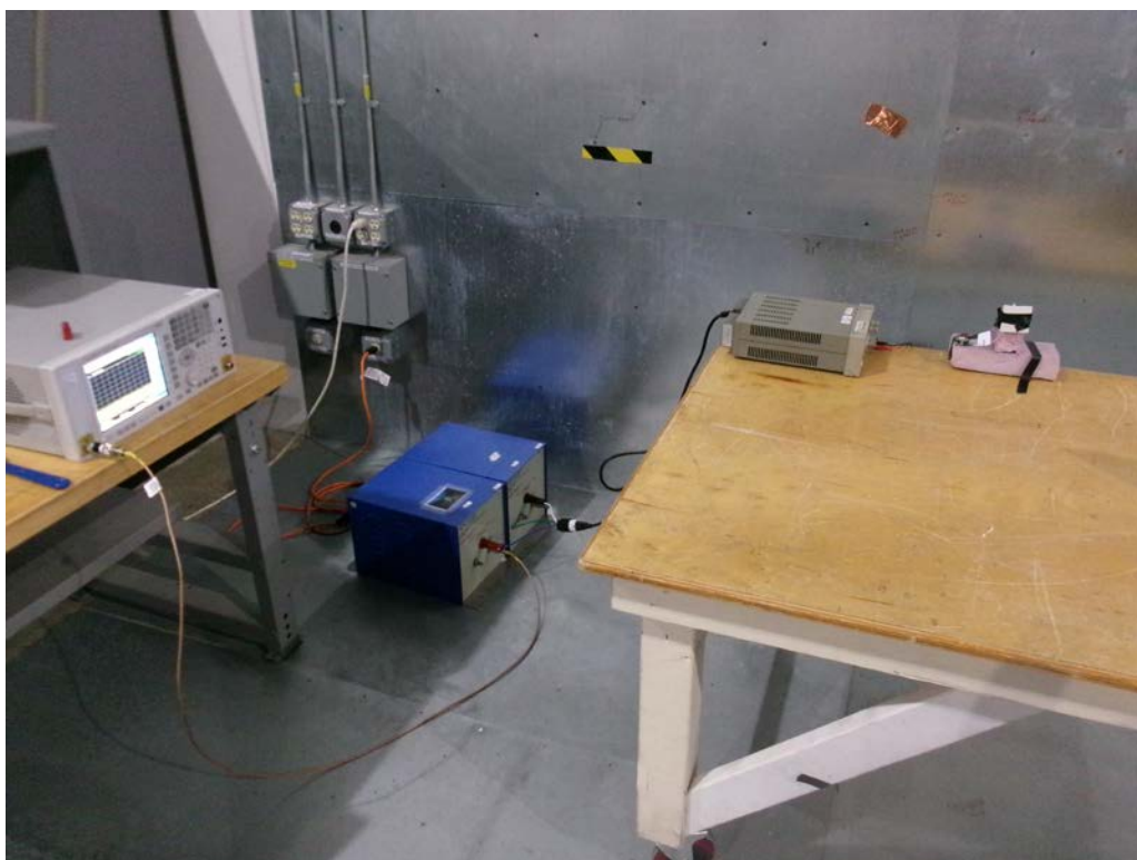
AC Line Conducted Emissions - AC Side of DC Supply
