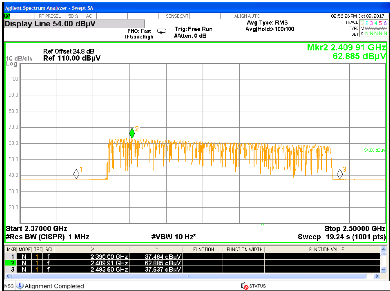
Figure 28: Radiated Emission at the Restricted Band Edge for Hopping Mode at DH5 – Horz. (Ave)
