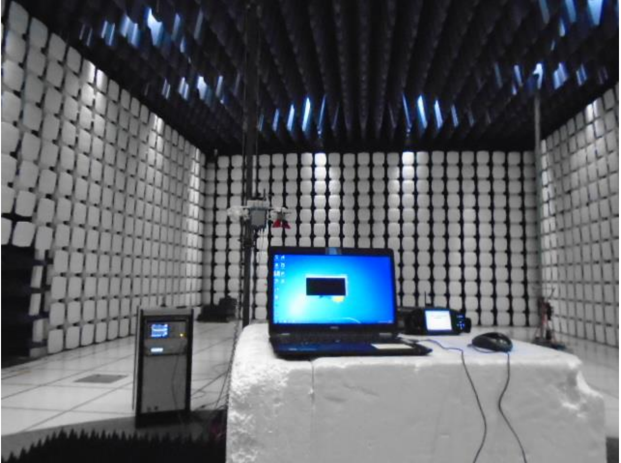
Figure 5: Test Setup for Above 1 GHz (Front View)
