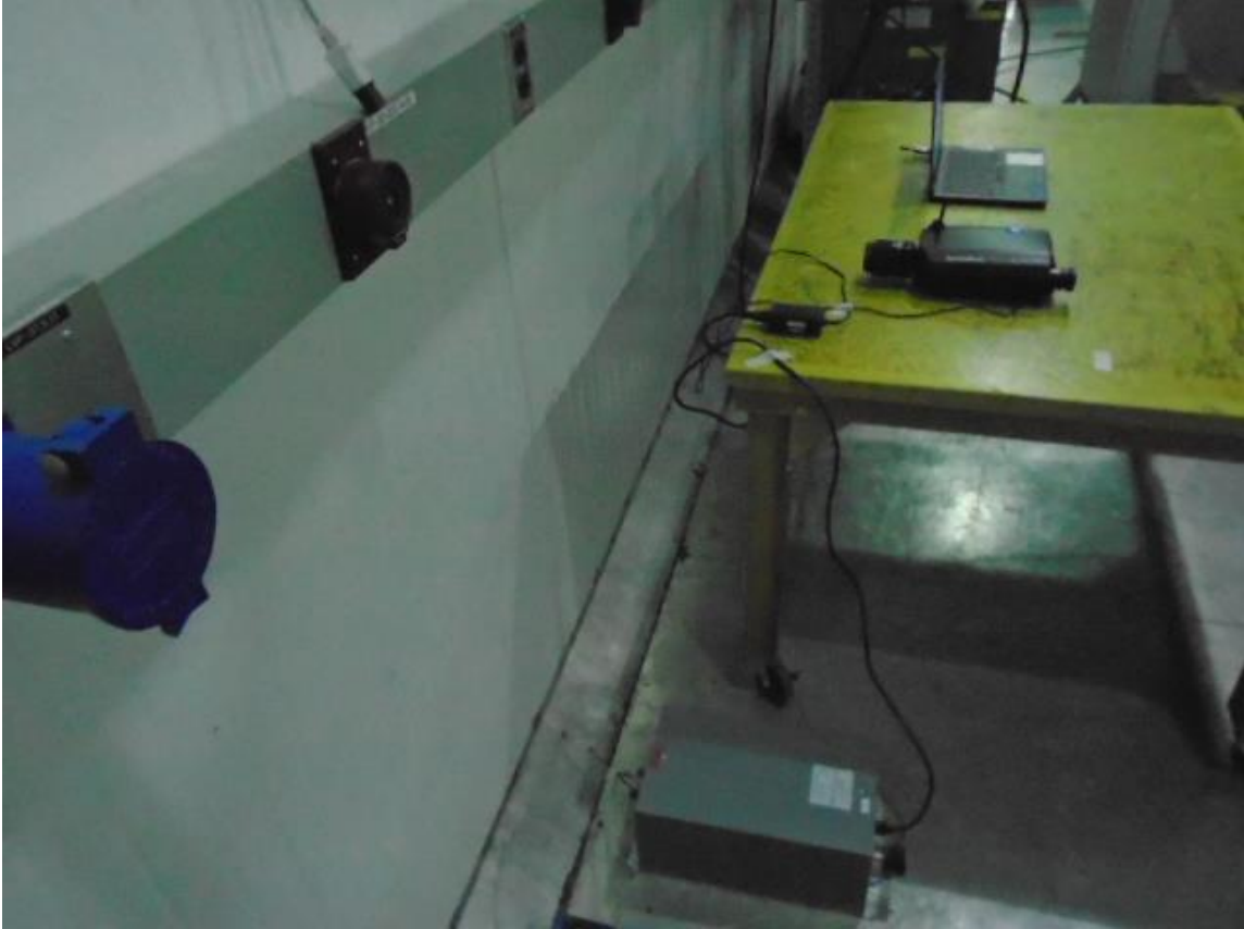
Figure 10: AC Conducted Emission Test Setup (Side)
