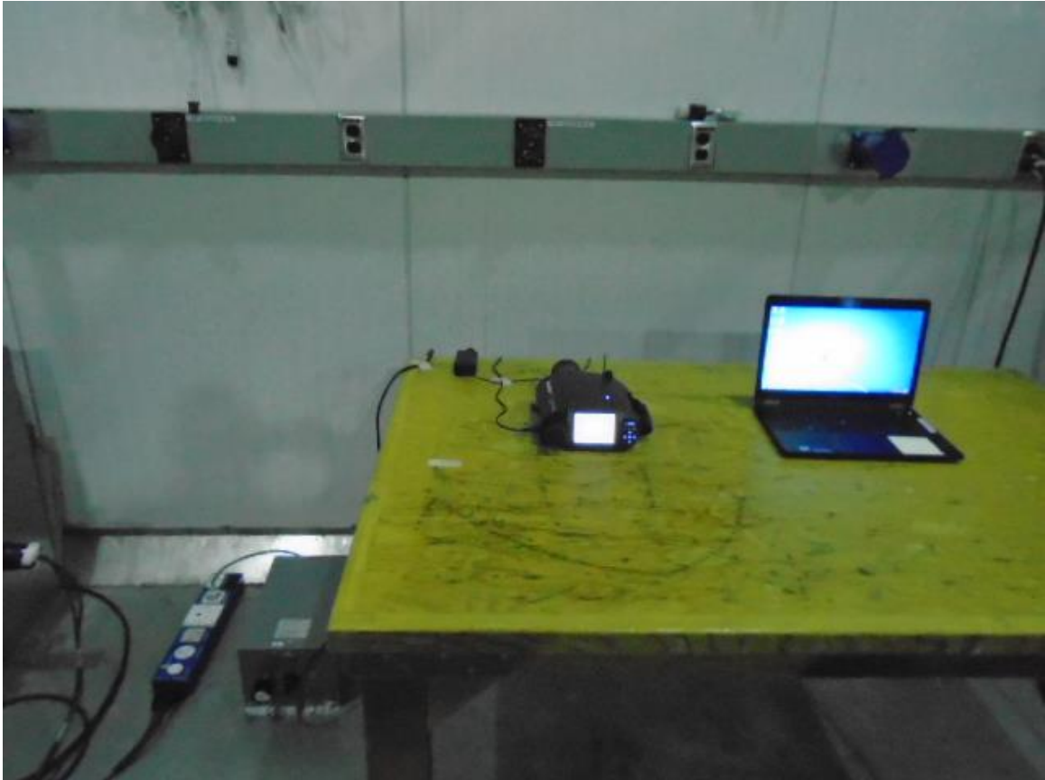
Figure 9: AC Conducted Emission Test Setup (Front)
