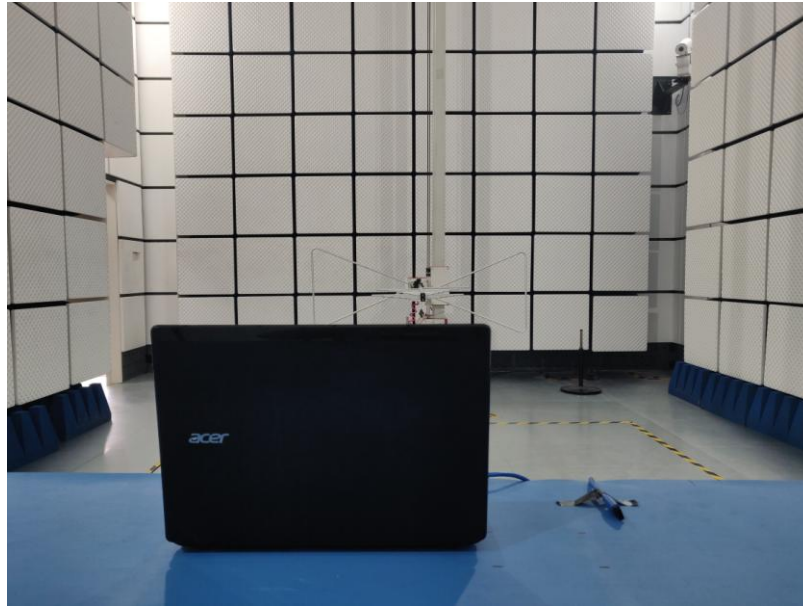
Radiated emission Test Setup-2 (30MHz~1GHz)
