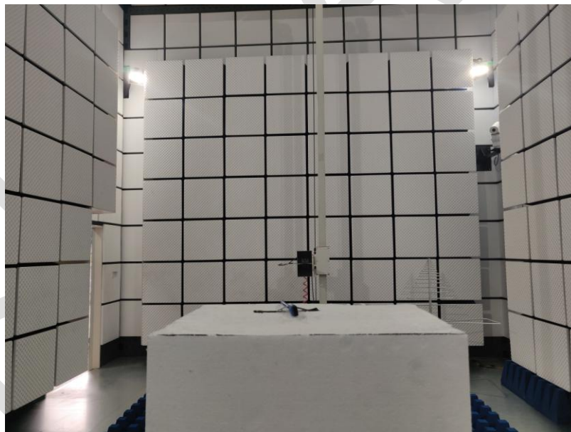
Radiated spurious emission Test Setup-3(Above 1GHz)
