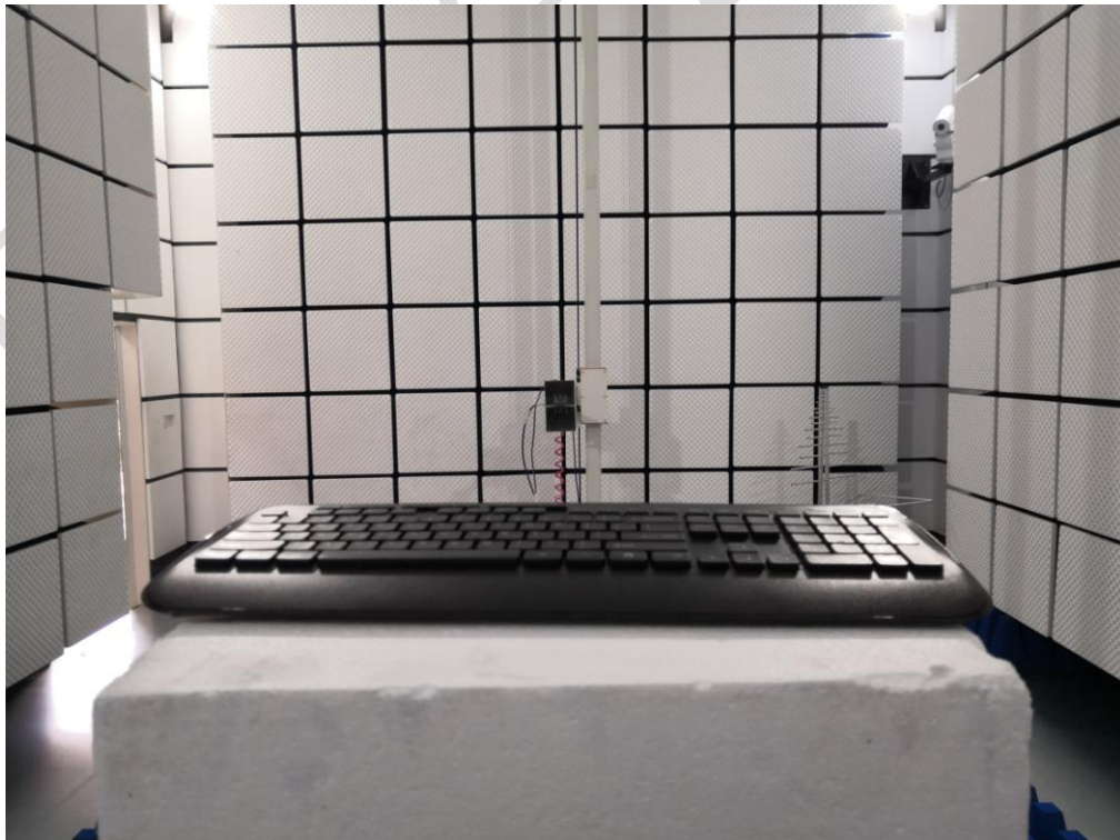
Radiated spurious emission Test Setup-3(Above 1GHz)
