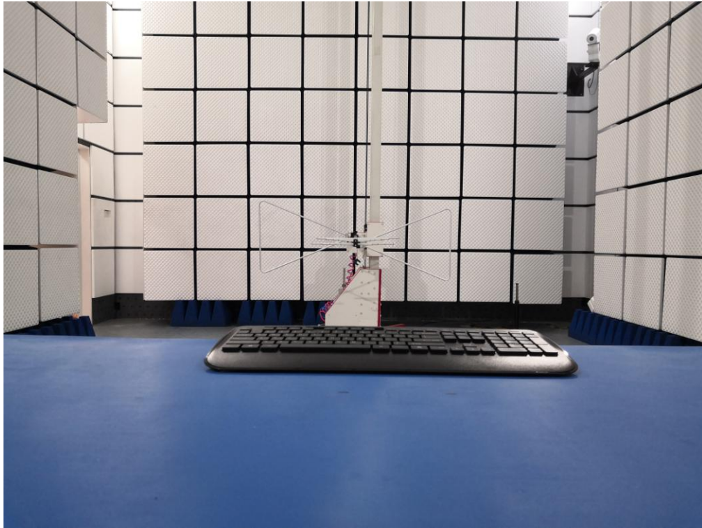
Radiated emission Test Setup-2 (30MHz~1GHz)
