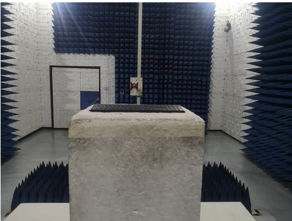
FCC RADIATED EMISSION TEST SETUP ABOVE 1GHZ
