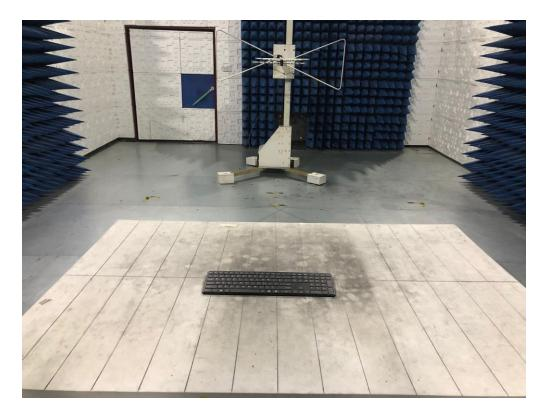
RADIATED EMISSION TEST SETUP ABOVE 1GHZ
