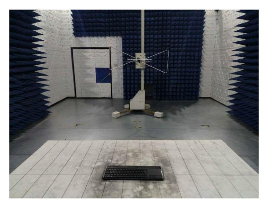
FCC RADIATED EMISSION TEST SETUP ABOVE 1GHZ
