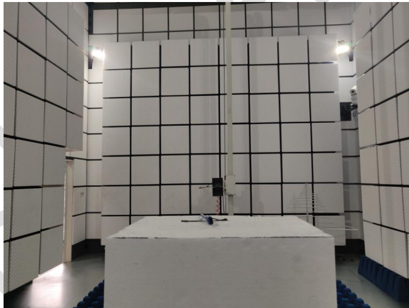
Radiated spurious emission Test Setup-3(Above 1GHz)
