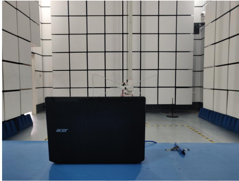
Radiated emission Test Setup-2 (30MHz~1GHz)
