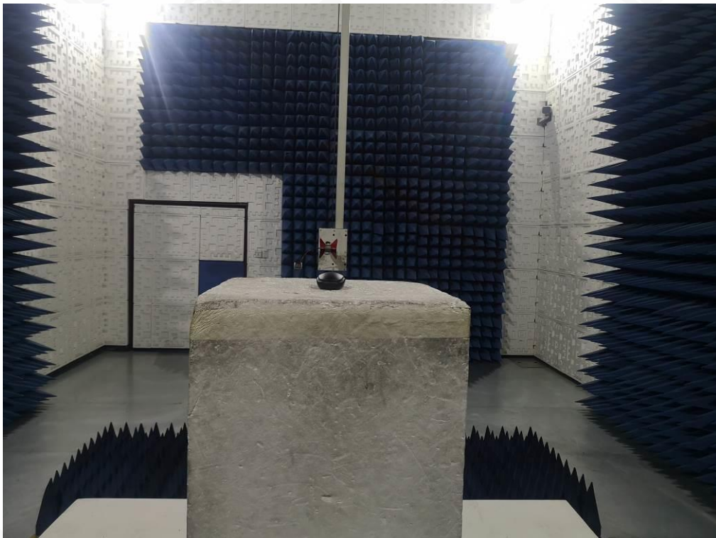
FCC RADIATED EMISSION TEST SETUP ABOVE 1GHZ
