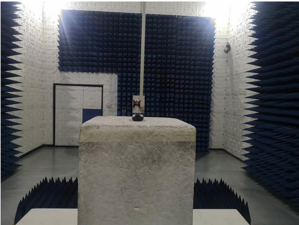
FCC RADIATED EMISSION TEST SETUP ABOVE 1GHZ
