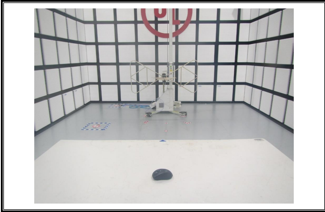
RADIATED RF MEASUREMENT SETUP (ABOVE 1 GHz- X axis)
