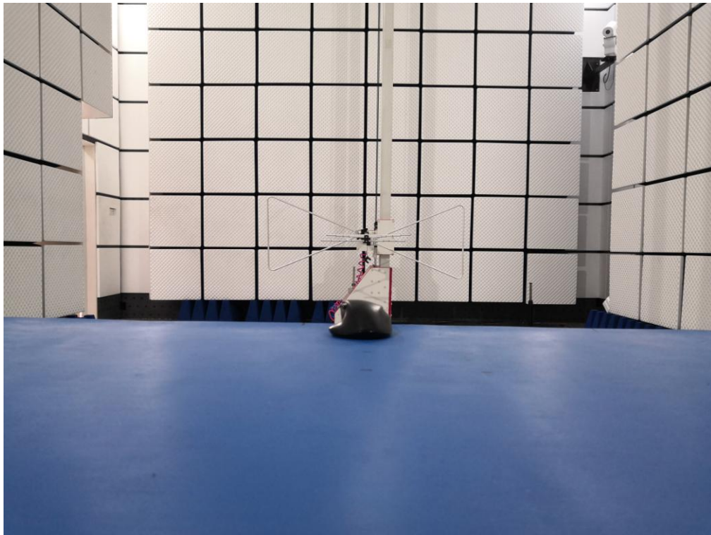
Radiated emission Test Setup-2 (30MHz~1GHz)
