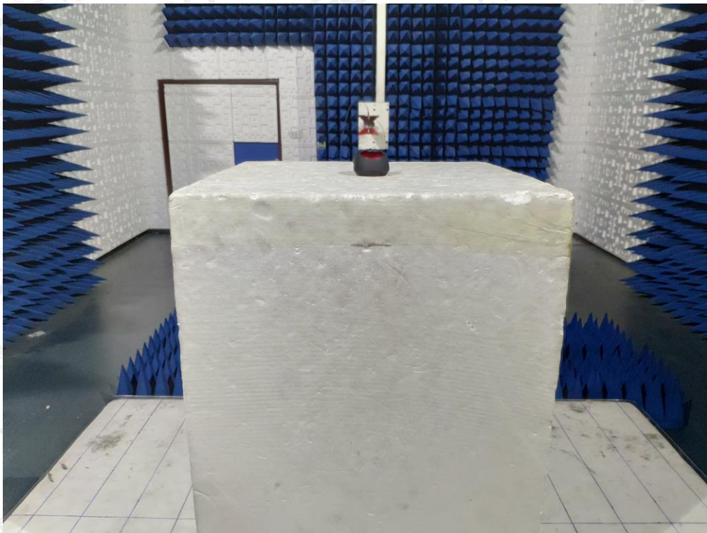
FCC RADIATED EMISSION TEST SETUP ABOVE 1GHZ
