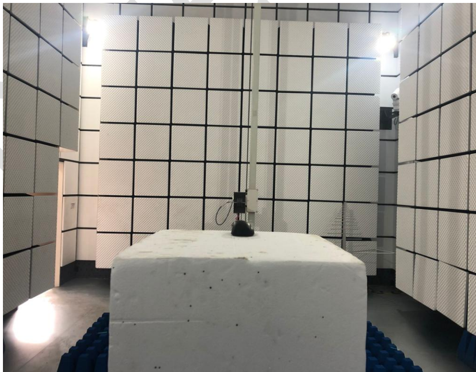
Radiated spurious emission Test Setup-3(Above 1GHz)
