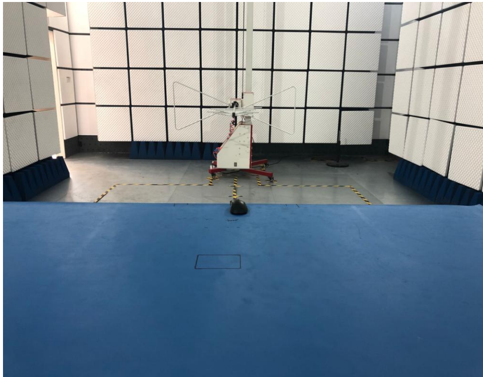
Radiated emission Test Setup-2 (30MHz~1GHz)
