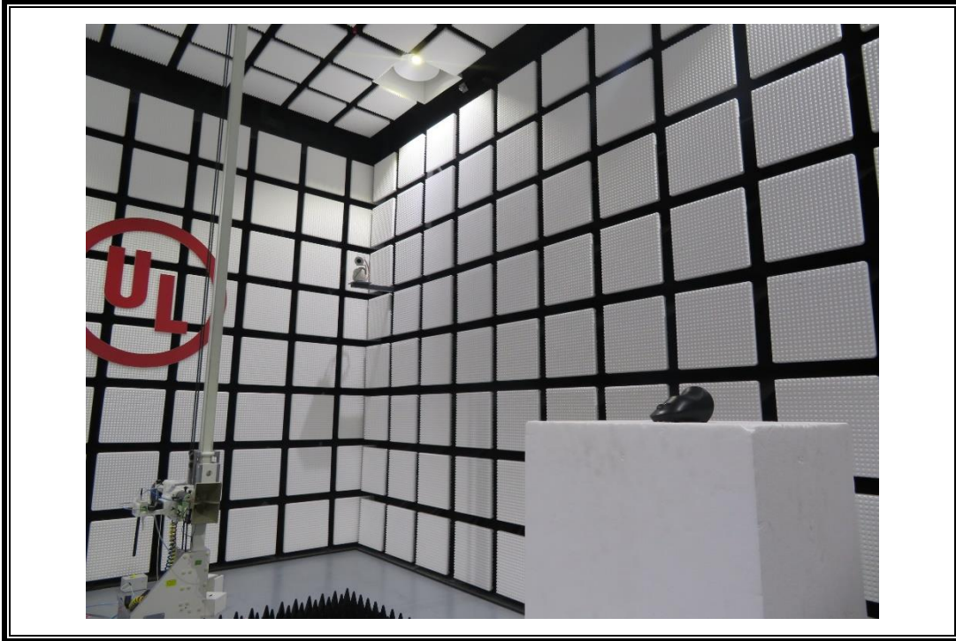
RADIATED RF MEASUREMENT SETUP (ABOVE 1 GHz- Y axis)
