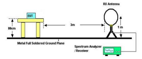
The setting of the spectrum analyzer
