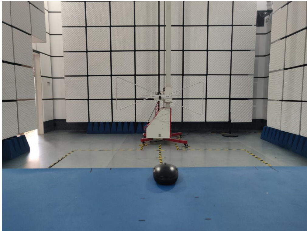
Radiated emission Test Setup-2 (30MHz~1GHz)
