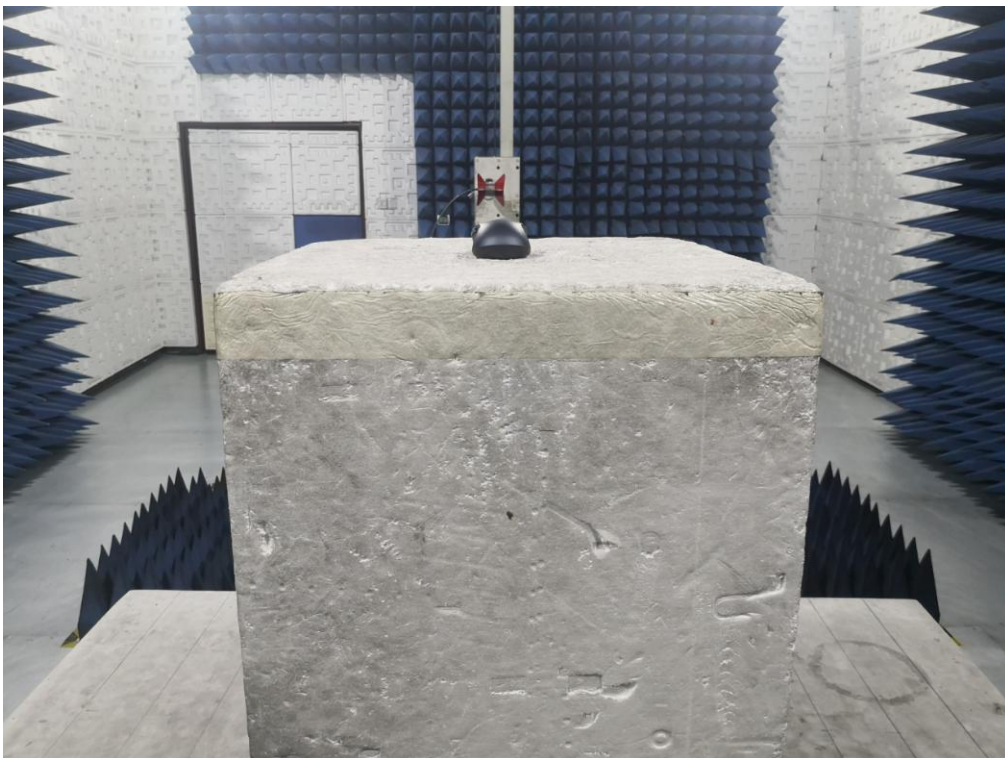
RADIATED EMISSION TEST SETUP ABOVE 1GHZ
