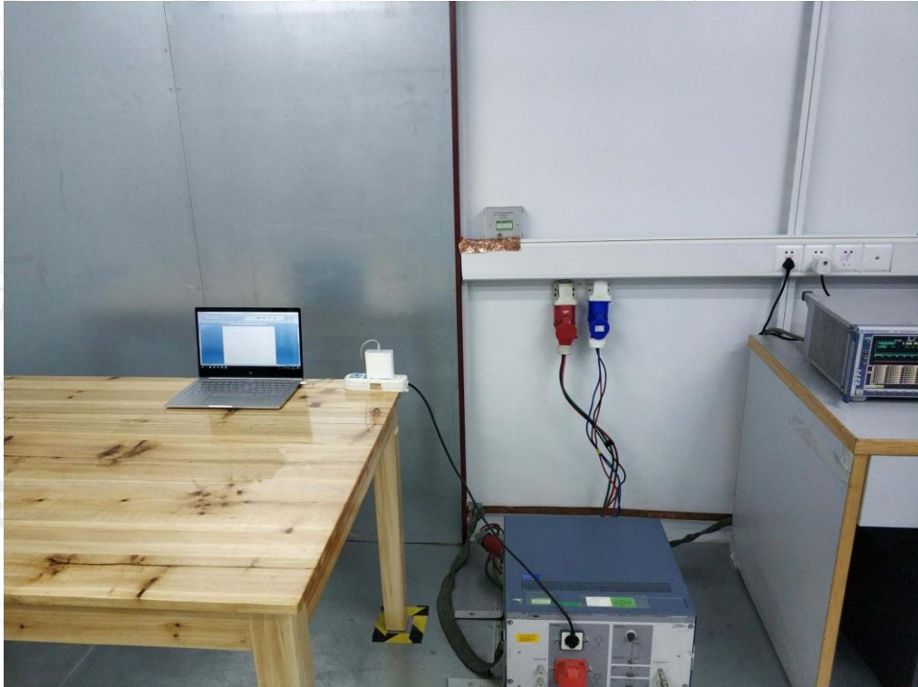
FCC RADIATED EMISSION TEST SETUP BELOW 1GHZ
