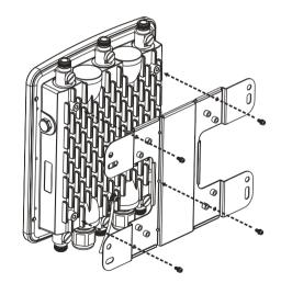
B) Determine which placement to be assembled. Drive the four round head screws to attach the Pole Mount Bracket to the bracket.
