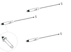
C) Place the lock and flat washers on the four cap screws and drive the screws to attach the bracket to the back of the Access Point.
