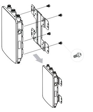
D) Attach the device onto the wall by tightening the bolt's flat washers and nuts to secure the bracket to the mounting surface.
