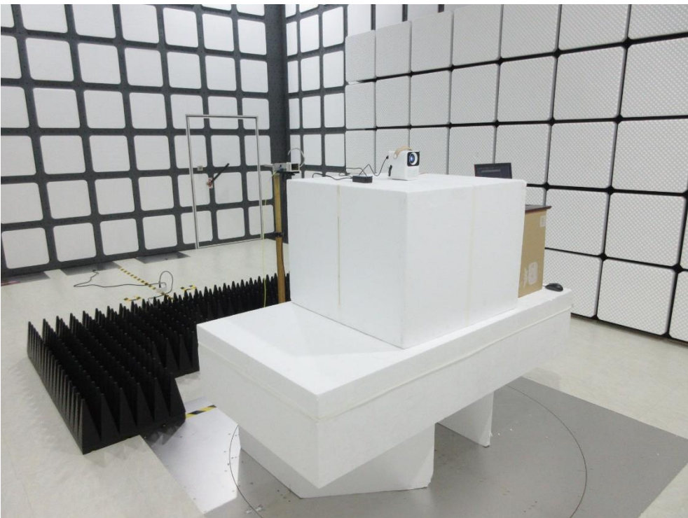
Description: Radiated Emission Test Setup for 18GHz~40GHz
