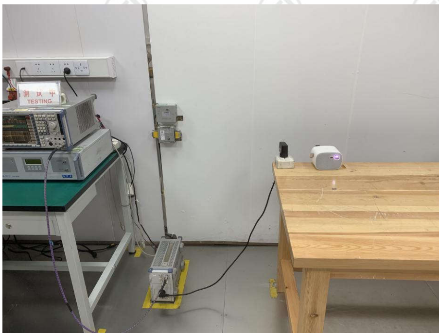
AC Power Line Conducted Emission
