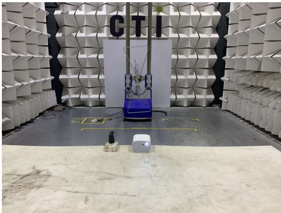
Radiated spurious emission Test Setup-1(Below 1GHz)
