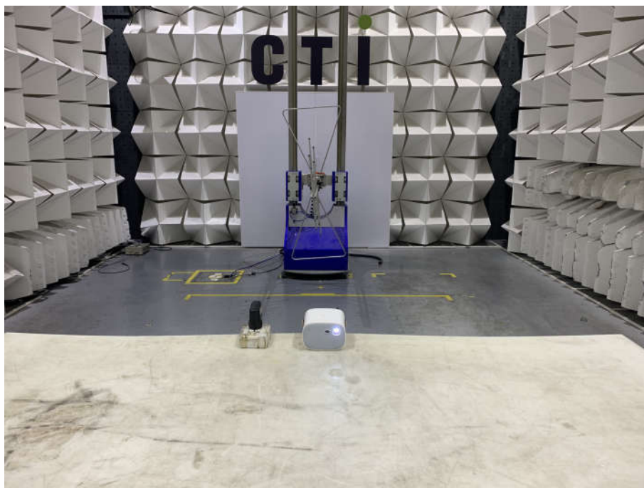
Radiated spurious emission Test Setup-1(Below 1GHz)
