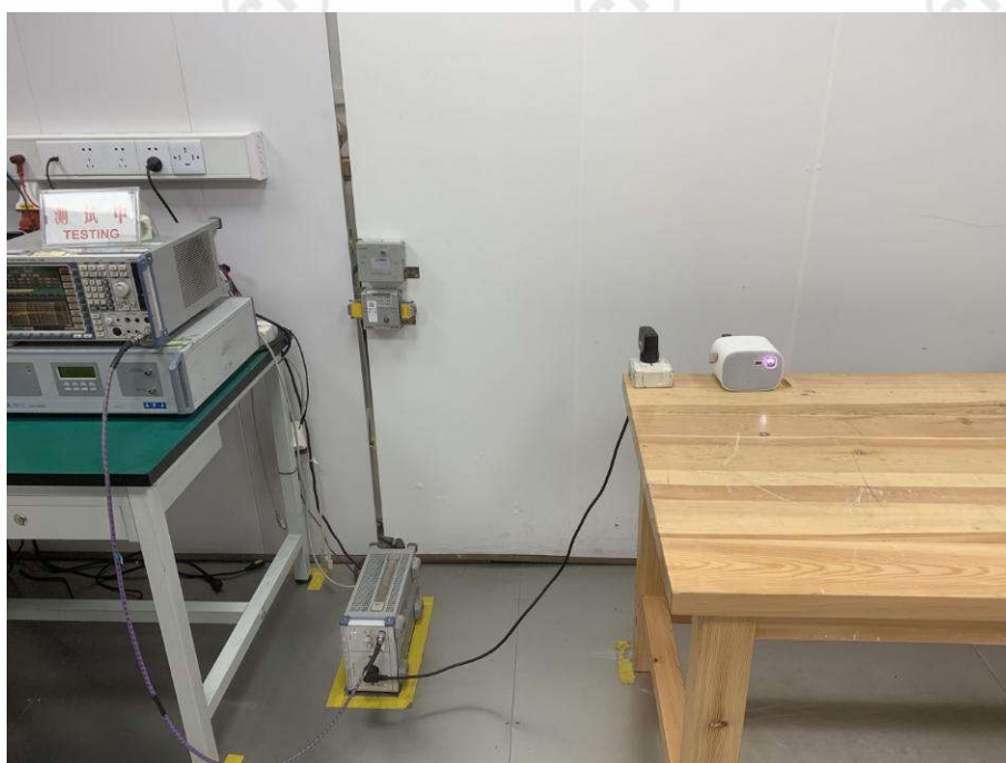
AC Power Line Conducted Emission
