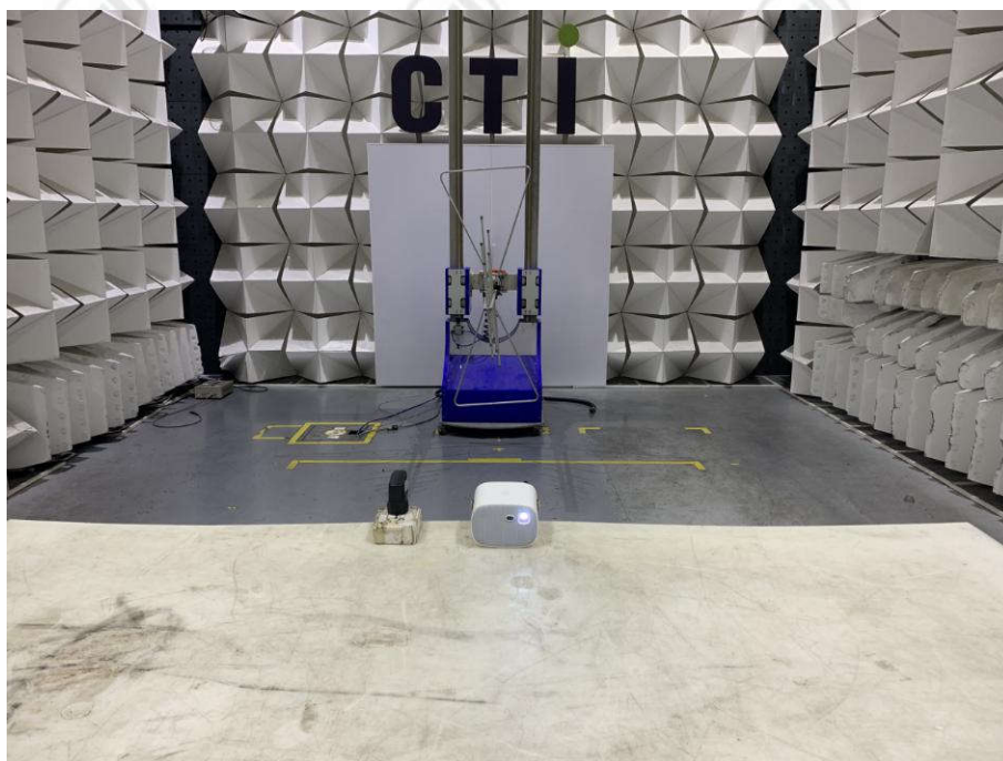
Radiated spurious emission Test Setup-1(Below 1GHz)
