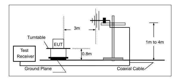
(C) For radiated emissions above 1000MHz
