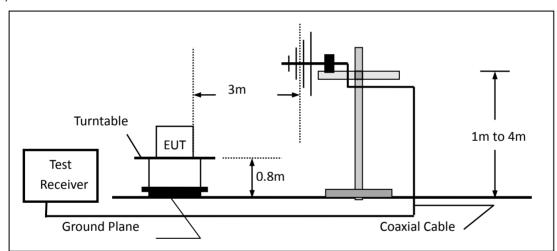
(c) For radiated emissions above 1000MHz
