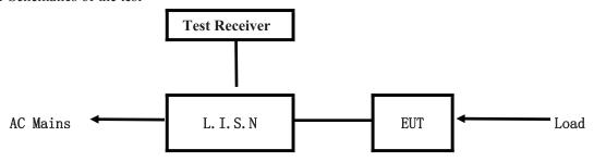
EUT: Equipment Under Test
