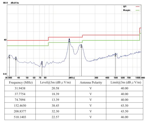
Note: Measurements were done at all three channels (high, middle, low), and the worst case (high channel) was submitted only. GFSK is the worse case.
