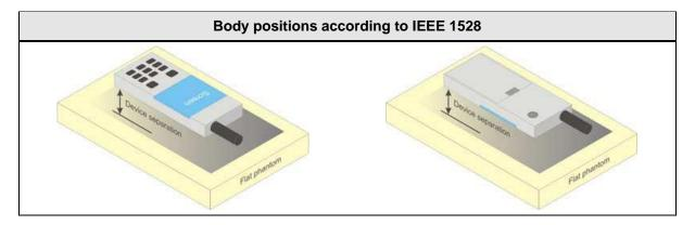
In body worn configuration the device is positioned parallel to the phantom surface with either top or bottom side of the EUT facing against the phantom.
