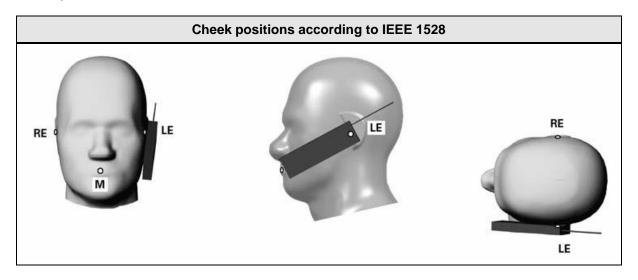
The handset is positioned close to the surface of the phantom such that point A is on the (virtual) extension of the line passing through points RE and LE on the phantom (see Figure), such that the plane defined by the vertical centerline and the horizontal line of the handset is approximately parallel to the sagittal plane of the phantom. Next the handset is translated towards the phantom along the line passing through RE and LE until handset point A touches the pinna at the ERP.
