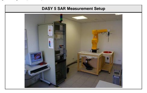
The following Diagram show the elements involved in the measurement setup.
