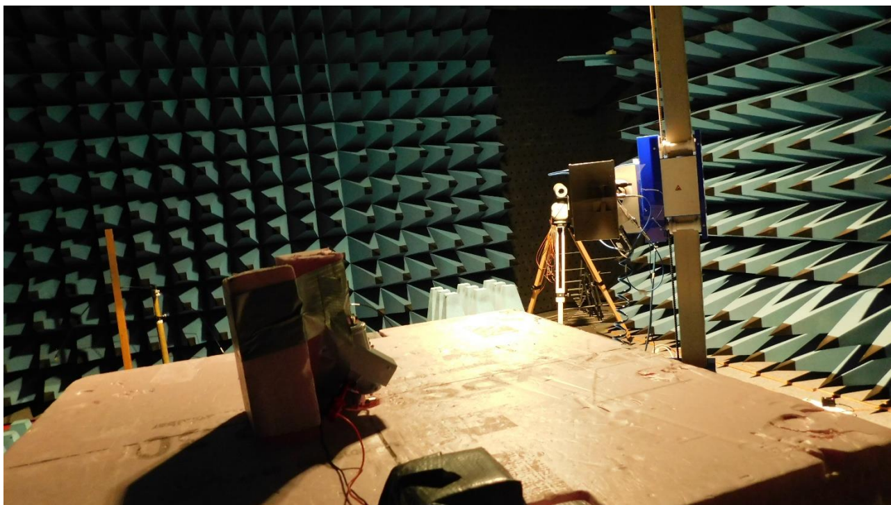
Picture 5: FS-SAC, radiated emission test 1 GHz – 17 GHz (front view)
