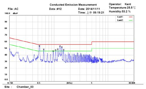
Condition: FCC Part 15 Class B Conduction (QP)
