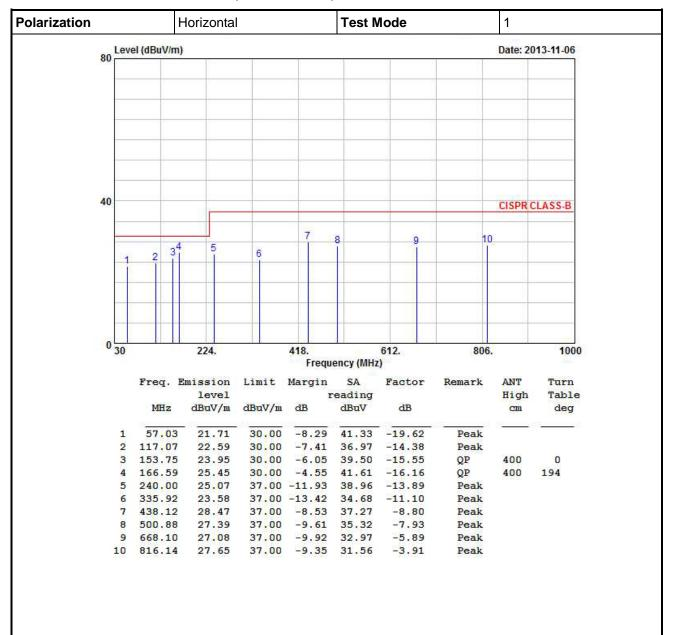
Note 1: Level (dBuV/m) = Read Level (dBuV/m) + Antenna Factor (dB) + Cable Loss (dB) - Preamp Factor (dB). 2: Over Limit (dBuV/m) = Limit Line (dBuV/m) - Level (dBuV/m).
