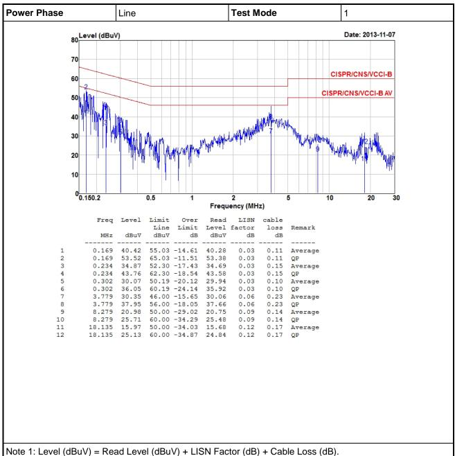
2: Over Limit (dBuV) = Limit Line (dBuV) - Level (dBuV).
