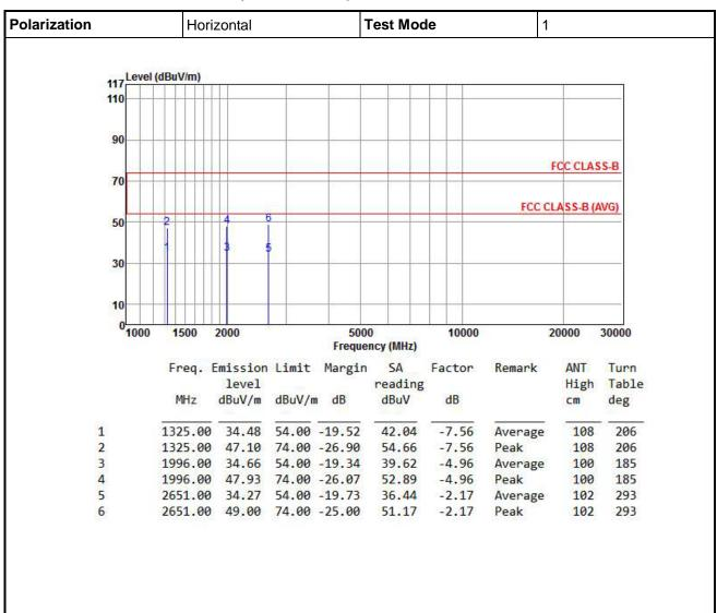
Note 1: Level (dBuV/m) = Read Level (dBuV/m) + Antenna Factor (dB) + Cable Loss (dB) - Preamp Factor (dB). 2: Over Limit (dBuV/m) = Limit Line (dBuV/m) - Level (dBuV/m).
