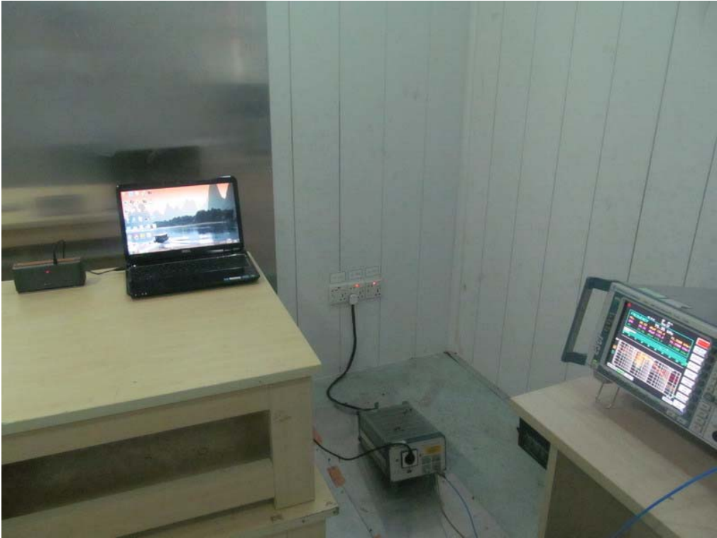
FCC RADIATED EMISSION TEST SETUP
