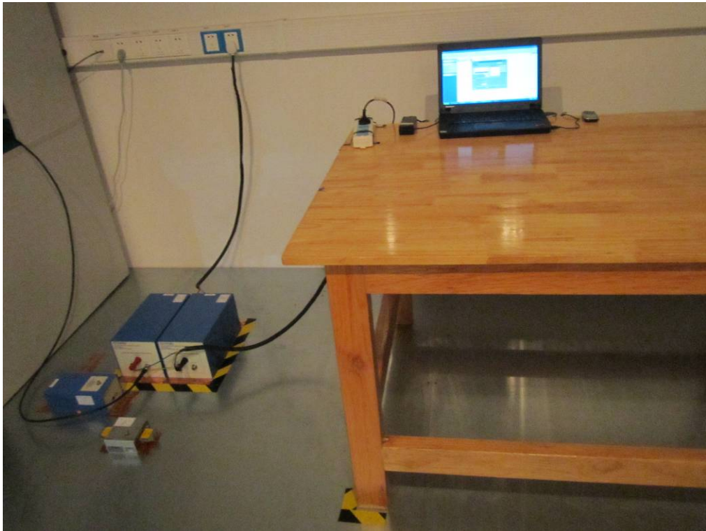
Conducted Emissions Test Setup Front View
