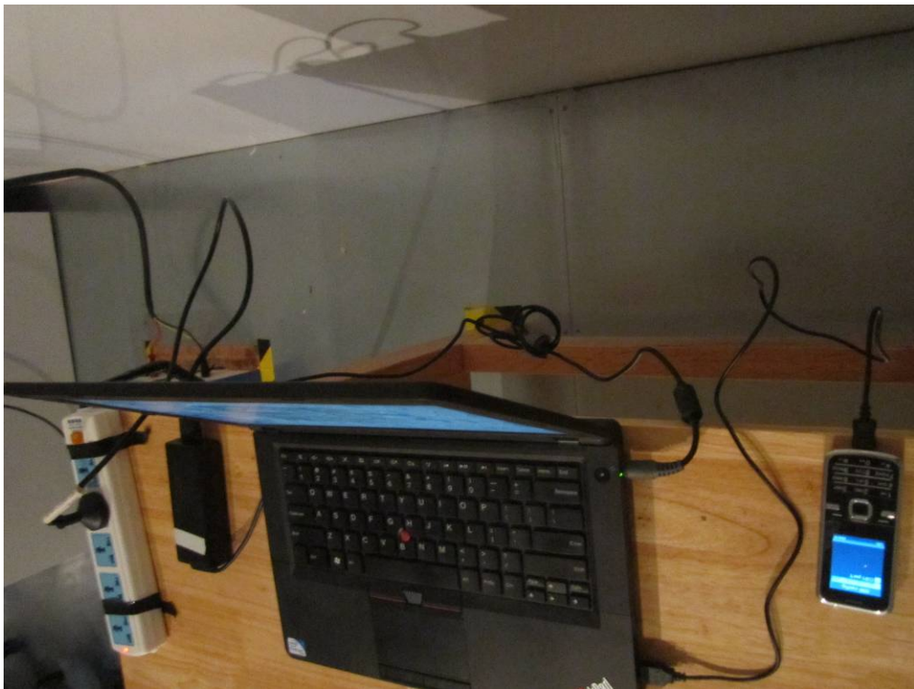
Conducted Emissions Test Setup Side View
