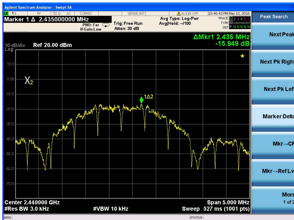
Power spectral density plot on channel 6
