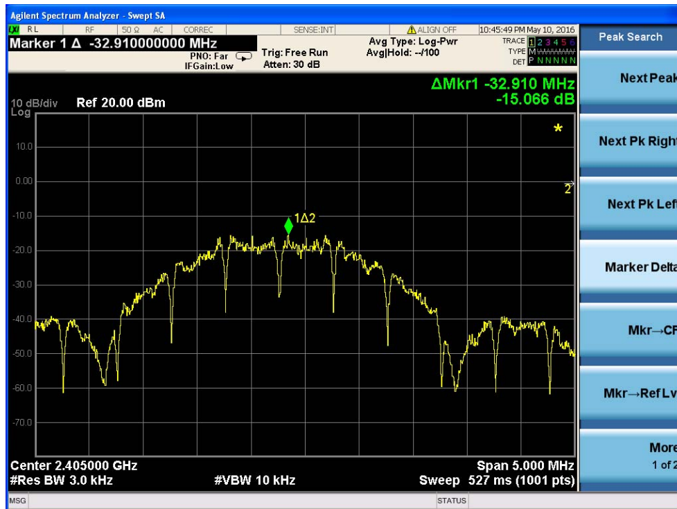
Power spectral density plot on channel 6
